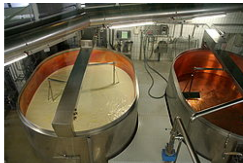
During industrial production of Emmental cheese, the as-yet-undrained curd is broken by rotating mixers.
