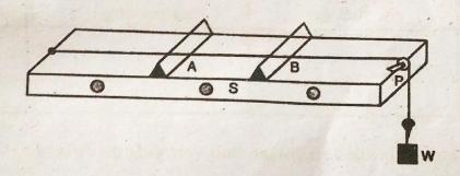
It consists of a thin metallic wire stretched across two movable bridges A and B on the top of a hollow, wooden sounding box (S') about one metre long. One end of the wire is fixed to a peg at one end of the box. The other end of the wire passes over a smooth fixed pulley (P) and carries a weight hanger W. The length of the vibrating segment of the wire can be altered with the help of the
