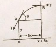
Consider a small segment AB of the displaced string (Figure). Its length is  $\delta x$ . The tension T in the string has the same magnitude everywhere. But the direction of T changes from point to point. The tensions at A and B will be tangential to the string at A and B. Let the tangent to the string at A make an angle  $\theta$  with the X-axis Component of the tension at A in the Y-direction is
