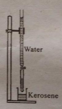
The interfacial tension  $\sigma$  between water and kerosene i calculated using the formula.
