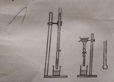
A short glass tube is connected to the lower end of a burette (or funnel) clamped vertically by means of a rubber tube (figure). The funnel is filled with the liquid whose surface tensions is to be determined. A beaker is arranged under the glass tube to collect the liquid dropping from the funnel. The stopcock is adjusted so
