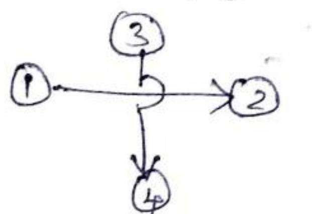
Common Errors in drawing a network!
